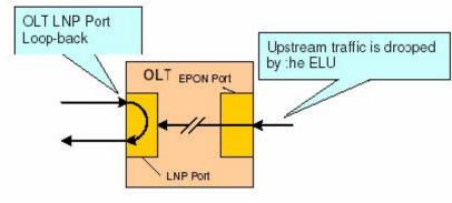
Figure 6: Uplink Port Loopback
