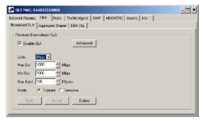
This command is identical to the functionality of the Link SLA Panel except that it is used to provision an SLA for the broadcast channel, as apposed to a unicast link. This unique feature of the OLT allows the OLT To use its large 40Meg buffer ram to serve the requirements of all ONUs, resulting in a 1:32 cost reduction (assuming 32 ONU deployment).
