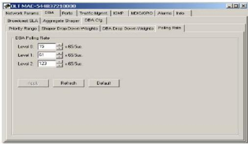
The polling rates panel allows the operator to configure the rate at which each link will be solicited to determine if it has any data to transmit. Smaller values result in lower latency and increased overhead. For priority 0, the scheduling latency is approximately equal to the larger of the polling rate and the cycle length.
