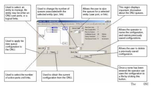
configuration panel allows the operator to change queue sizes and save configurations.
