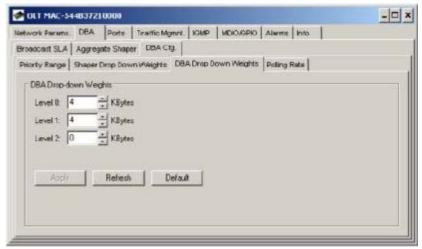
DBA drop down weights are used by the DBA to reserve bandwidth for each priority level. This allows the OLT to fix the latency and reserve a percentage of bandwidth for links in each priority level. The drop down weight for priority level n  $\mathbf{MUST}$  be greater than or equal to the provisioned DBA Weight for all links in priority level n+1.
