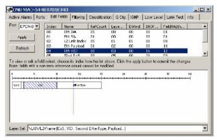
The TK3701/TK3711 and future ONUs support highly configurable line rate classification engines. Depending on the model, the ONU lookup engine is capable of simultaneously examining anywhere from 8-12 fields in the frame! The position and size of each field is programmed into the lookup engine prior to use in filtering and classification rules.
